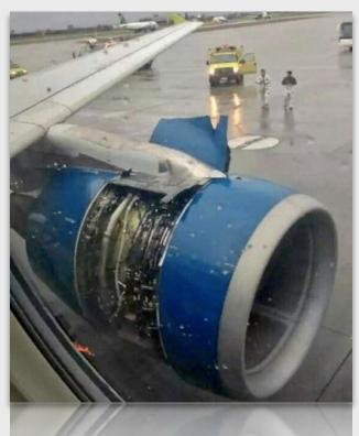
The investigation showed that prior to departure, the No.1 engine cowlings were opened by maintenance crew to check the oil levels of the Integral Drive Generator (IDG) and the filter differential pressure indicator. After this was completed, the cowlings were closed but not locked. The captain performed the walk around check but did not notice this.
